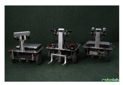
Figure 1.3: The three Robolabs robots using the RoboEx platform. The central robot, in addition to the rest of devices, has mounted a forklift
