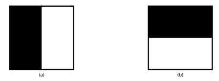
**Figure 2.24**. Haar wavelet filters to compute the responses in *x* (a) and y direction (b). The dark parts have the weight -1 and the light parts +1.
