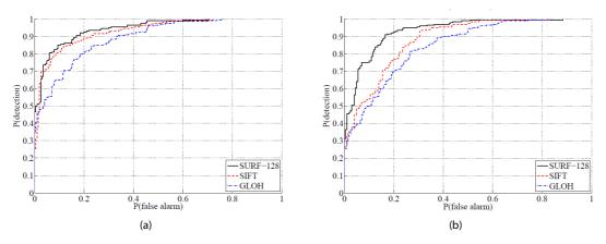
**Figure 3.11**. Comparison of different descriptor strategies for a naive Bayes classifier working on a bag-of-words representation. Top: descriptors evaluated on random edge pixels. Bottom: on SURF keypoints.
