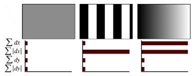
**Figure 2.28**. The descriptor entries of a sub-region represent the nature of the underlying intensity pattern. Left: In case of a homogeneous region, all values are relatively low. Middle: In presence of frequencies in x direction, the value of  $\Sigma |dx|$  is high, but all others remain low. If the intensity is gradually increasing in x direction, both values  $\Sigma |dx|$  and  $\Sigma |dx|$  are high.
