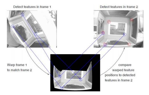
Figure 3.2. Repeatability is tested by checking if the same real-world features are detected in different views. A geometric model is used to compute where the features reproject to.
