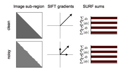
Figure 3.7. Due to the global integration of SURF's descriptor, it stays more robust to various image perturbations than the more locally operating SIFT descriptor.
