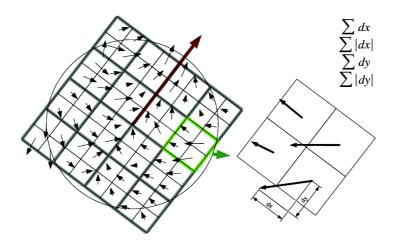
**Figure 2.27**. To build the descriptor, an oriented quadratic grid with  $4\times4$  square sub-regions is laid over the interest point (left). For each square, the wavelet responses are computed. The  $2\times2$  sub-divisions of each square correspond to the actual fields of the descriptor. These are the sums dx, |dx|, dy, and |dy|, computed relatively to the orientation of the grid (right).
