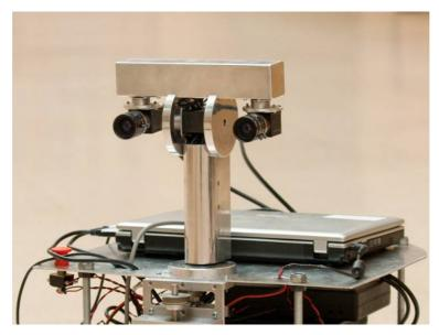
Figure 1.4: RoboLab robots use stereo cameras to estimate its position through visual odometry (among others approaches).
