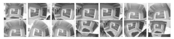
Figure 3.3. Box dataset: photographs taken of a test rig (consisting of photographs pasted to the inside of a cuboid) with strong changes of perspective, changes in scale and large amounts of radial distortion. This tests the corner detectors on planar textures.
