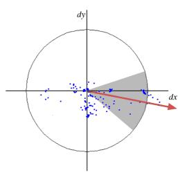
**Figure 2.25**. Orientation assignment: A sliding orientation window of size  $\pi/3$  detects the dominant orientation of the Gaussian weighted Haar wavelet responses at every sample point within a circular neighborhood around the interest point.
