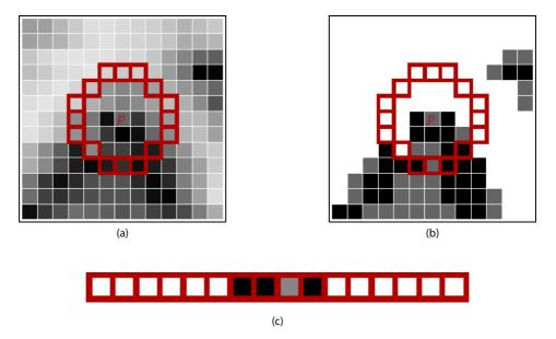
**Figure 2.14**. Over a candidate pixel *p* (a), the pixels of the Bresenham circumference are clasified in one of the three sorts: darker (in black), similar (in gray) and brighter (in white) (b). In (c) the pixels of the circumference are showed as a row.
