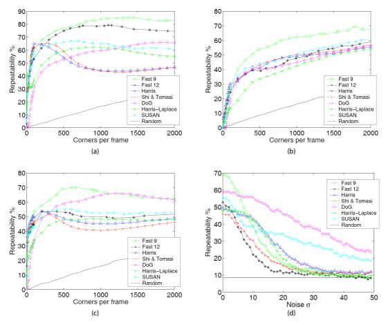
**Figure 3.6**. (a), (b), (c): Repeatability results for the three datasets as the number of features per frame is varied. (d): repeatability results for the bas-relief data set (500 features per frame) as the amount of Gaussian noise added to the images is varied. For FAST and SUSAN, the number of features can not be chosen arbitrarily; the closest approximation to 500 features per frame achievable is used.
